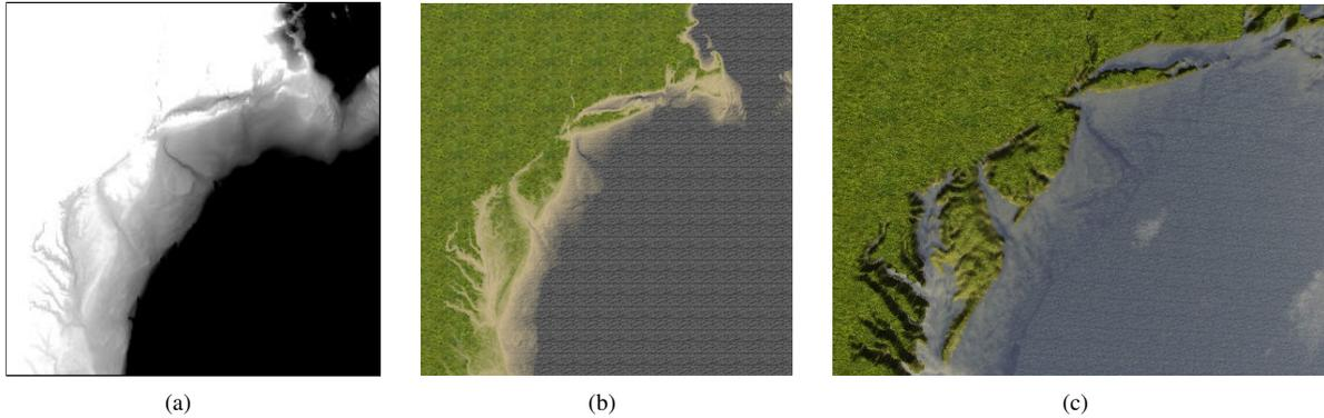
Fig. 1. A heightmap (a), generated from NGDC’s ETOPO1 model, is used to create a texture (b) for the 3D object (c) of the terrain in SimGUI.
