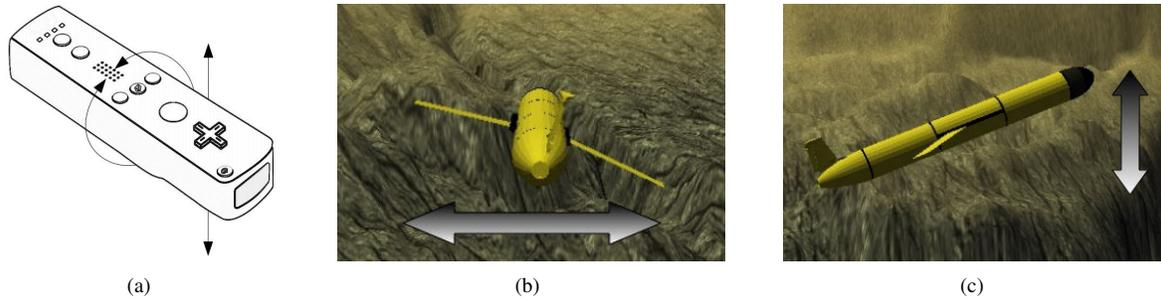
Fig. 2. The Wii Remote has been integrated with SimGUI to control a virtual Slocum Glider. The roll of the remote (a) translates to a roll on the vehicle (b). Likewise, the glider’s pitch (c) is defined by the pitch of the controller (a).
