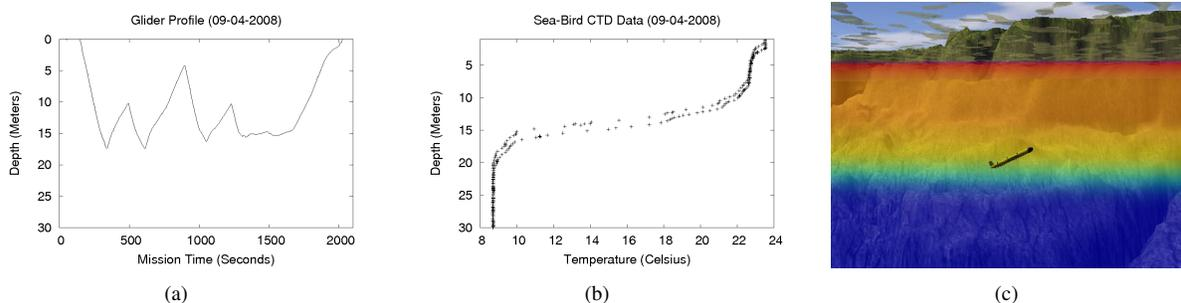
Fig. 4. A flight profile of a Slocum Glider tracking a thermocline (a) in a water column as measured in (b). The water column and the flight of the vehicle can be displayed for analysis in SimGUI (c).
