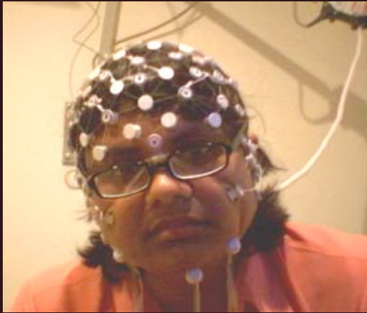
High-density 64 sensor array
