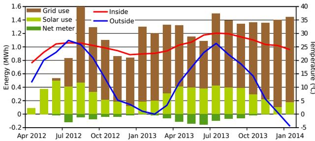
**Figure 2.** Energy consumption, net metering, and temperatures from April 2012 to January 2014.
