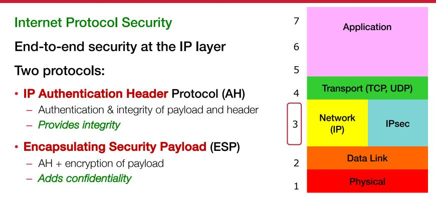
IPsec is a separate protocol from UDP or TCP – protocols 50 (ESP) & 51 (AH) in the IP header. Layer 3 protocol – gateway routers are responsible for encapsulating/decapsulating
