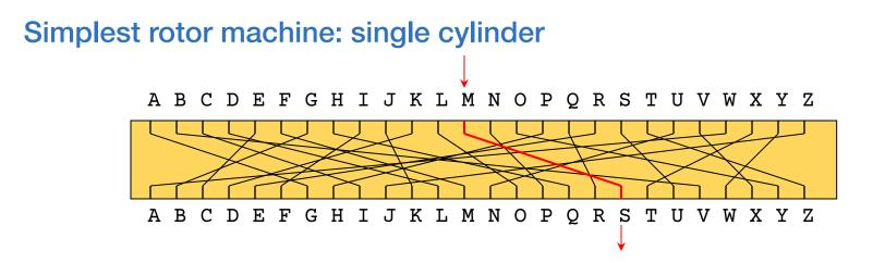
After a character is entered, the cylinder rotates one position
