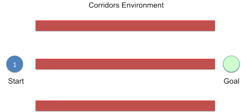
Figure 2: The environment from the prototypical motion coordination example. It contains two least-cost homotopic classes of paths, each corresponding to a different corridor.
