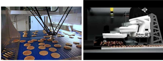
Fig. 1. Examples of robots deployed in industrial settings tasked to arrange objects in desired configurations through pick and place: (left) ABB's IRB 360 FlexPicker rearranging pancakes; (right) Stäubli's TP80 Fast Picker robot.
