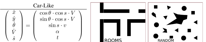
Fig. 10. The state update equations for the car-like vehicles and scenes “rooms” and “random”.
