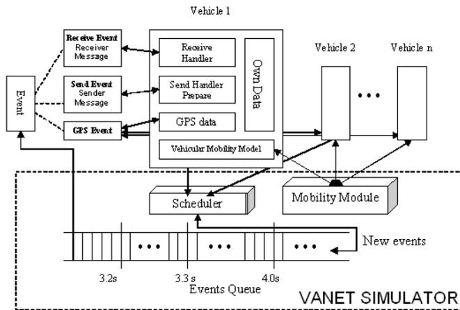
Figure 1 : Simulator architecture
