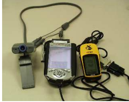
Figure 9: Prototype Node with Video Camera and GPS Receiver Attached
