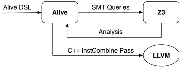
Figure 3: The figure illustrates how the optimization in Alive domain specific language (DSL) is checked for correctness by the Alive interpreter with queries to the Z3 (SMT) solver. On successful verification, the Alive interpreter generates the C++ code for use in LLVM. If the verification is unsuccessful, it generates counter examples with concrete values to illustrate the error.
