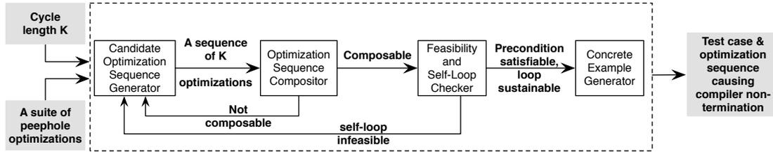
Figure 2: Workflow of our termination checking algorithm.
