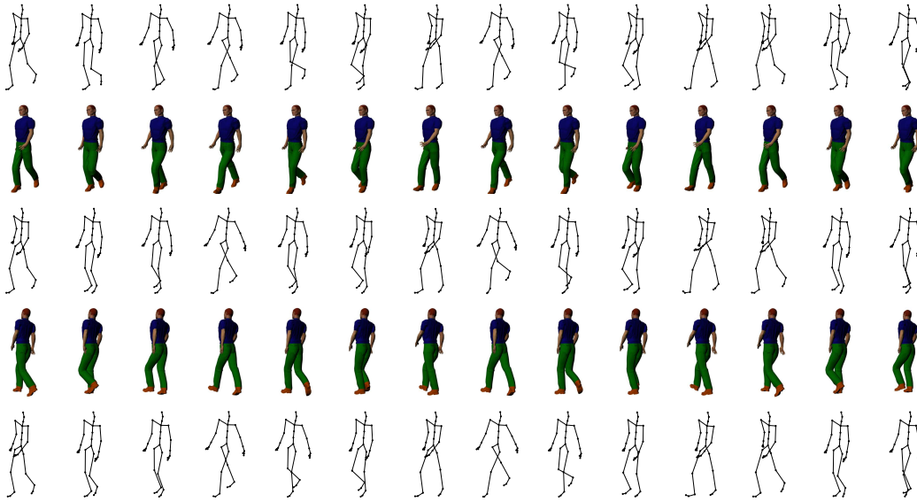
Figure 6. Input images with unknown view point and 3D reconstructions using DPLSA tracking. First row: true pose. Second and third rows: \frac{\pi}{4} view angle. Fourth and fifth rows: \frac{3\pi}{4} view angle.
