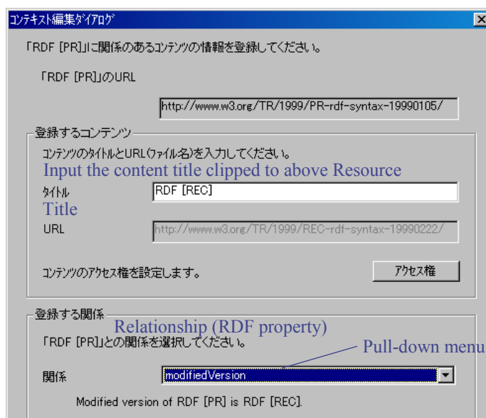
Figure 8. A dialog window for adding meanings of relationships when content is clipped
