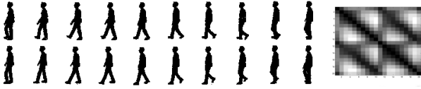
Figure 1. Twenty sample frames from a walking cycle from a side view. Each row represents half a cycle. Notice the similarity between the two half cycles. The right part shows a plot of the distance between the samples. The two dark line parallel to the diagonal shows the similarity between the two half cycles.
