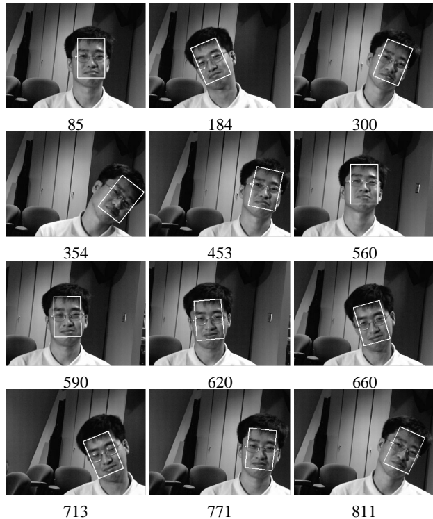
Figure 4. Tacking a Face: recovering translation and rotation in a closed-form for over 800 frames.
