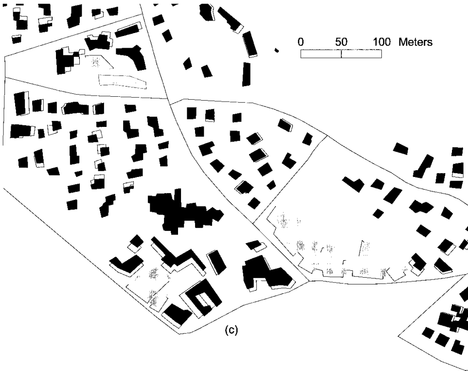
Figure 5(c). Example of the effect of including displacement cost. (c) Result obtained when displacement cost is taken into account; unnecessary displacement has been reduced.
