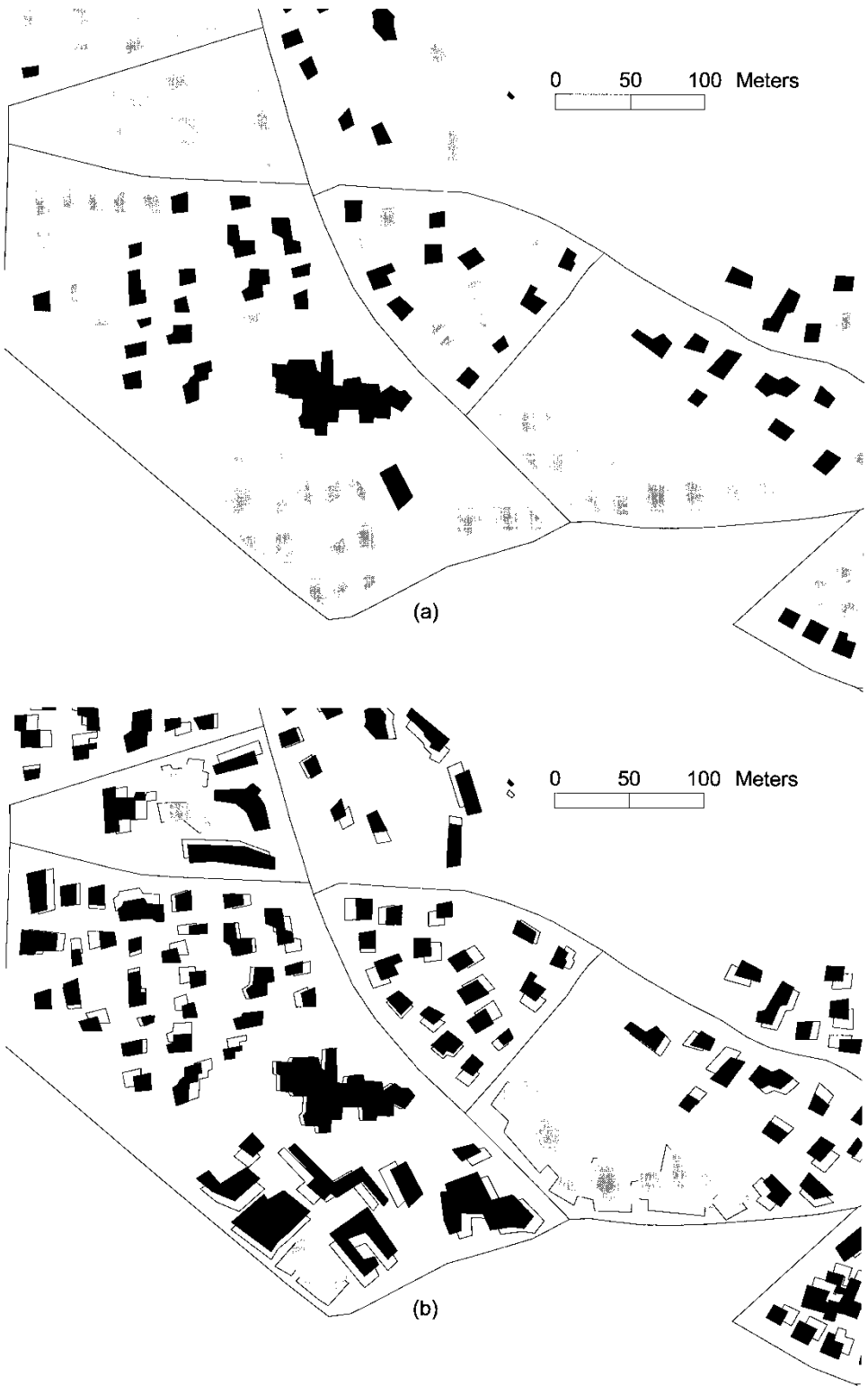
Figure 5(a-b). Example of the effect of including displacement cost. (a) Original data. (b) Result obtained without consideration to displacement cost (original object locations shown in background).
