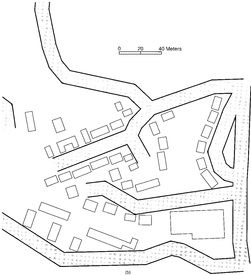
Figure 10(b). Large scale OS data example. (b) Graphic conflict resolved by application of displacement, size enlargement, size reduction and deletion.
