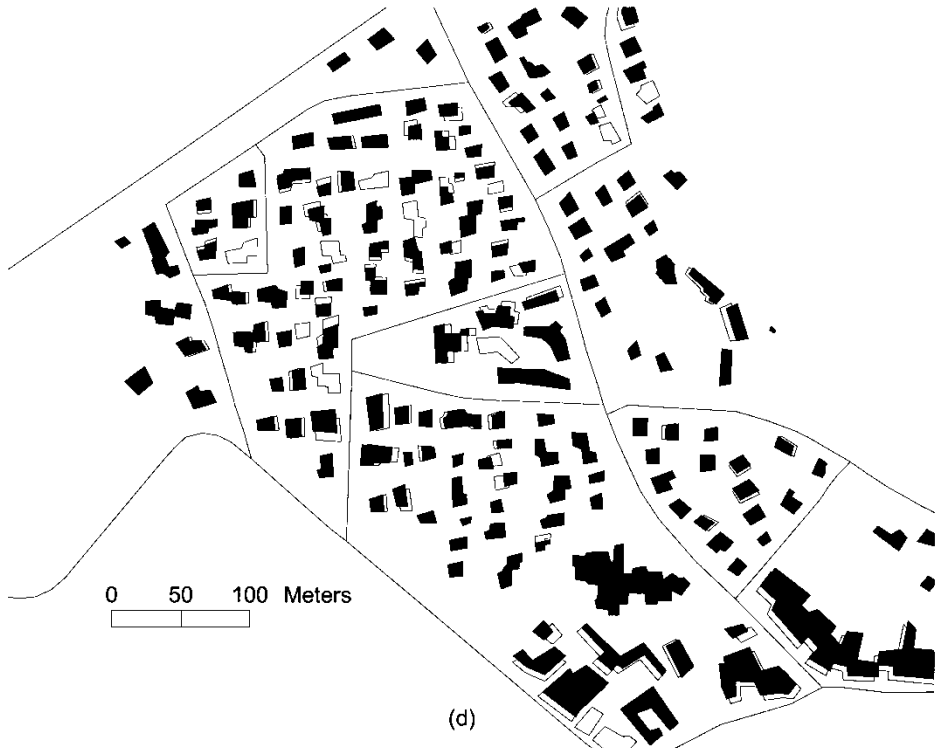
Figure 6(c-d). Application of deletion operator. (c) Deletion cost set too low, over-deletion. (d) A more appropriate deletion cost setting.
