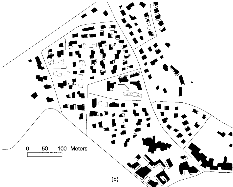
Figure 6(a-b). Application of deletion operator. (a) Original data. (b) Deletion cost set too high, not all spatial conflict removed.
